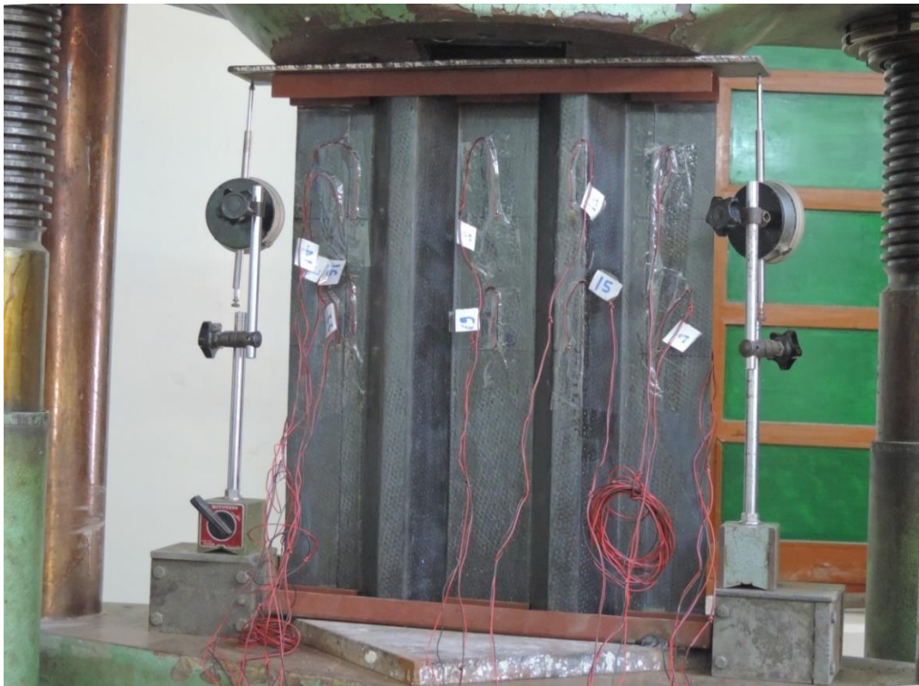
Figure 5.4 Specimen of hat-stiffened panel installation.
