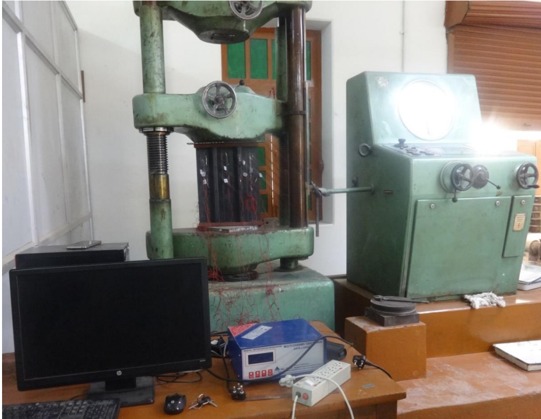
Figure 5.3 Experimental set up of hydraulic machine with strain gauge data-logger system.
