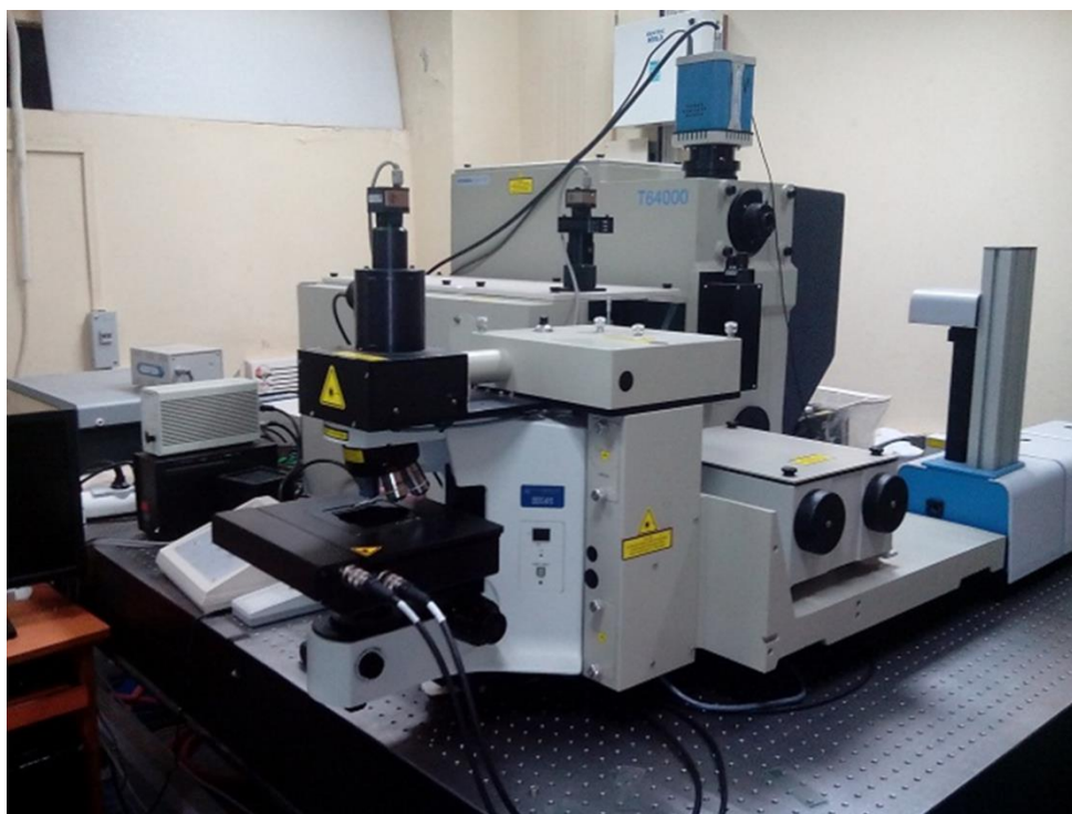
Figure 2.9 Experimental set-up used for Raman Measurement. (CRF IIT Kharagpur).
