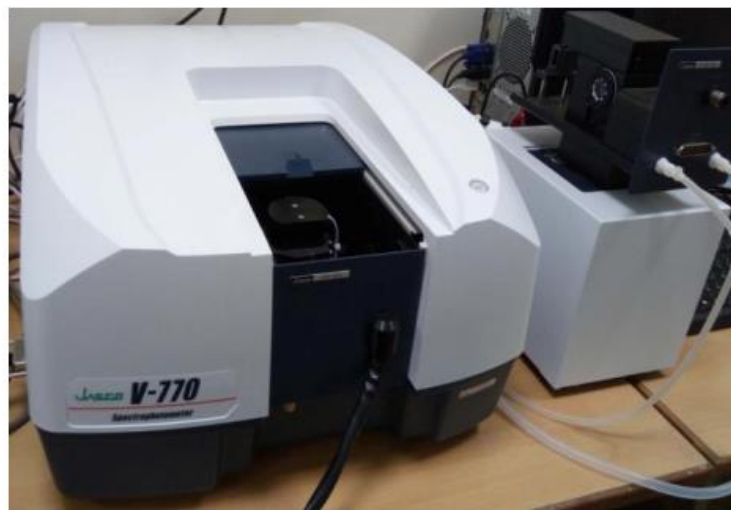
Figure 2.17 Experimental Set-up for UV-Vis measurement (IIT BHU).
