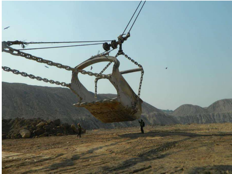
Figure 1. 3: A large dragline bucket
