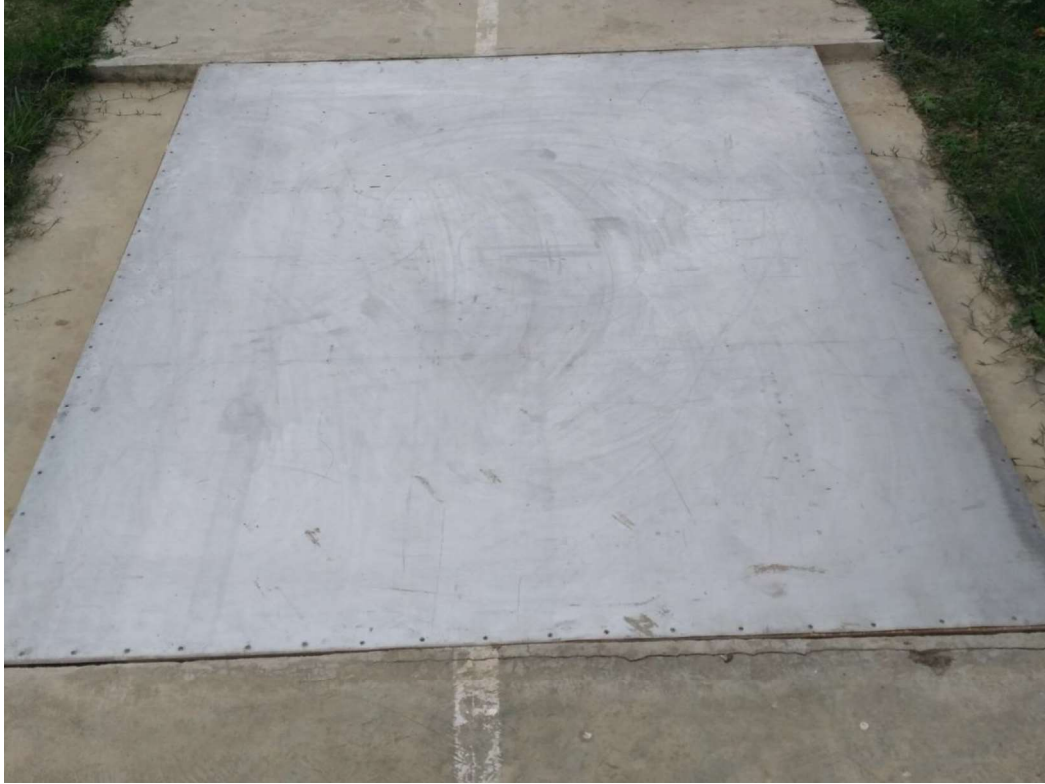
Figure 2.2 Aluminum sheet used during the calibration of the system
