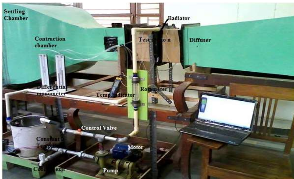
Figure 5.9: Photograph of the fully instrumented radiator experimental setup in wind tunnel
