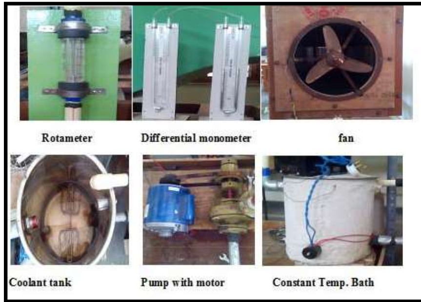
Figure 5.7: Other components for the radiator experimental setup
