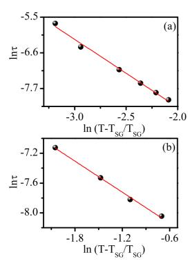
FIG. 7.  $\ln \tau$  vs  $\ln(T-T_{SG}/T_{SG})$  plot for (a) SG1 and (b) SG 2 transitions. Solid line shows the least squares fit for power law.
