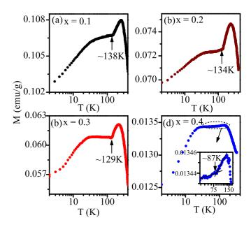
FIG. 20. The variation of ZFC magnetization of BF-xBT with temperature below 300 K measured at a field of 500 Oe for compositions (a) x=0.10, (b) 0.20, (c) 0.30, and (d) 0.40.
