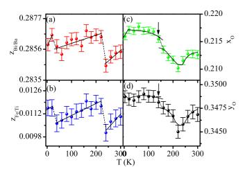
FIG. 16. Temperature dependence of the fractional z coordinates of (a) Bi/Ba and (b) Fe/Ti. The x and y coordinates of O are shown in (c) and (d). All these coordinates were obtained from the Rietveld refinements using neutron powder diffraction data.
