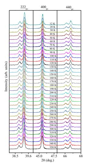
FIG. 11. The evolution of x-ray powder diffraction profiles of the  $(222)_{pc}$ ,  $(400)_{pc}$ , and  $(440)_{pc}$  reflections of BF-0.20BT with temperature showing absence of any structural phase transition.
