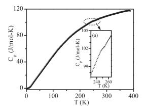
FIG. 4. The variation of specific heat capacity with temperature for BF-0.20BT. Inset (a) is a magnified view around SG1 transition depicting an anomaly.
