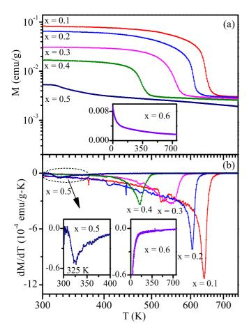
FIG. 18. (a) The variation of ZFC magnetization with temperature measured at a field of 500 Oe for various compositions in the range  $0.10 \le x \le 0.60$ . (b) shows the first derivative of M(dM/dT) with respect to temperature for these compositions.
