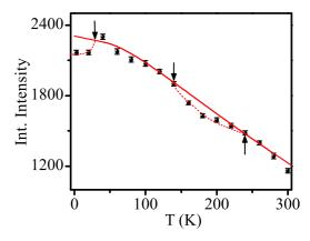
FIG. 15. Temperature-dependent variation of the integrated intensity of the AFM peak (111) (the miller indices are with respect to a doubled pseudocubic cell). Solid line is fit for Brillouin function.
