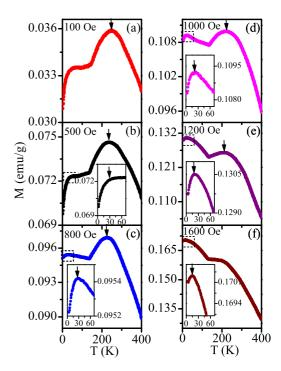
FIG. 8. ZFC dc magnetization vs temperature plots of BF-0.20BT measured at different applied fields. Insets depict the magnified view around SG2 transition.
