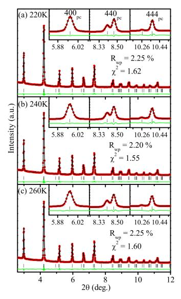
FIG. 12. Observed (filled circles), calculated (continuous line), and difference (bottom line) profiles obtained from the Rietveld refinement using SXRD data at (a) 220, (b) 240, and (c) 260 K using *R3c* space group for BF-0.20BT. The vertical tick marks above the difference profile represent the Bragg peak positions.
