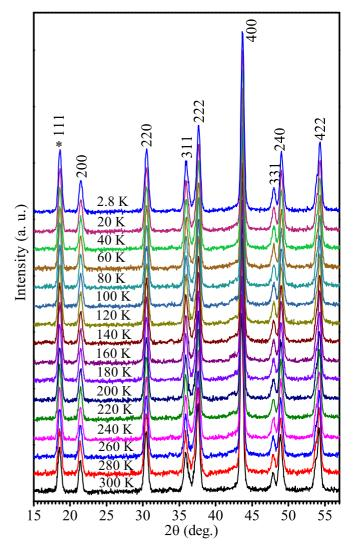
FIG. 14. The evolution of the neutron powder diffraction patterns with temperature in the limited  $2\theta = 15^{\circ} - 57^{\circ}$  range. The first peak is due to AFM ordering. The Miller indices are written with respect to a doubled pseudocubic cell.
