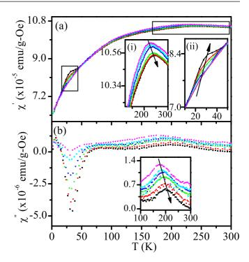
FIG. 5. Variation of  $\chi'(\omega, T)$  and  $\chi''(\omega, T)$  in the temperature range 2–300 K at various frequencies [47.3 ( $\blacktriangleright$ ), 97.3 ( $\blacktriangleleft$ , 197.3 ( $\blacktriangledown$ ), 297.3 ( $\blacktriangle$ ), 397.3 ( $\bullet$ ), and 497.3 ( $\blacksquare$ ) Hz]. Insets (i) and (ii) depict  $\chi'(\omega, T)$  on a zoomed scale for SG 1 and SG 2, respectively.
