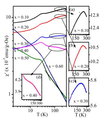
FIG. 19. (Left) The variation of  $\chi'(\omega, T)$  of BF-xBT with temperature at 497.3 Hz frequency for various compositions in the range  $0.10 \le x \le 0.60$ . Right panel [(a)–(c)] as well as (d) depict the zoomed view around the SG1 transition.
