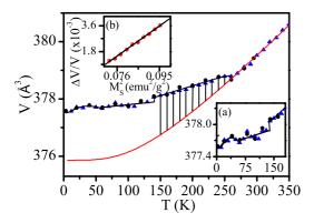
FIG. 13. Variation of unit cell volume with temperature: XRD ( $\blacktriangle$ ) and NPD ( $\bullet$ ) data. Solid line ( $\blacksquare$ ) is fit for Debye Grüneisen equation  $T_{\rm SG1}$ . Inset (a) shows the zoomed view around 140 K and SG2 transitions. Inset (b) depicts the variation of volume strain ( $\Delta V/V$ ) against square of magnetization ( $M_S^2$ ) obtained by M-H loop.
