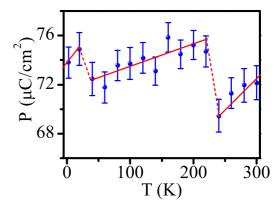
FIG. 17. Temperature-dependent variation of the spontaneous polarization calculated from the positional coordinates.
