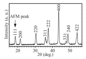
FIG. 3. Neutron powder diffraction pattern at room temperature. Arrow marks the antiferromagnetic peak. All the indices are written with respect to a doubled pseudocubic cell.
