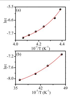
FIG. 6.  $\ln \tau \text{ vs } 1/T$  plot for (a) SG1 and (b) SG2 transitions. Solid line is the least squares fit for Vogel-Fulcher law.
