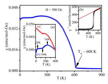
FIG. 1. ZFC dc magnetization vs temperature plot for an applied field of 500 Oe. Insets depict (a) the temperature dependence of dc magnetization under ZFC and FC conditions and (b) Curie-Weiss plot for BF-0.20BT above  $T_{\rm N}$ .
