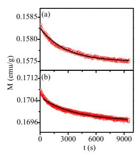
FIG. 10. Variation of thermoremanent remnant magnetization [M(t)] with time at (a) 200 and (b) 10 K for BF-0.20BT.
