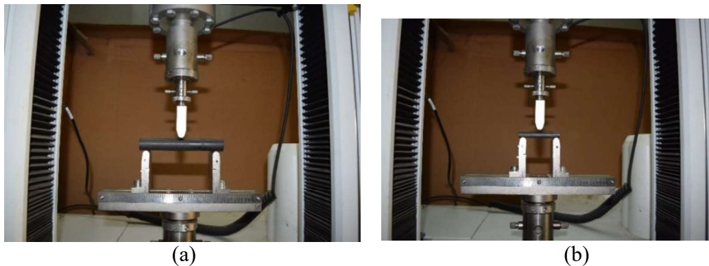
Fig. 5.17 Three point flexure assembly for (a) large, (b) small bimodular cylindrical graphite specimens
