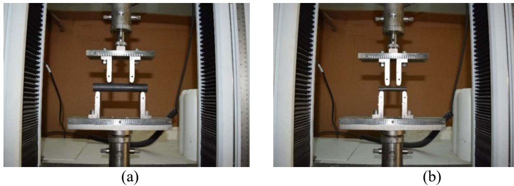
Fig. 5.19 Four point 1/4 loading flexure assembly for (a) large, (b) small bimodular cylindrical graphite specimens.
