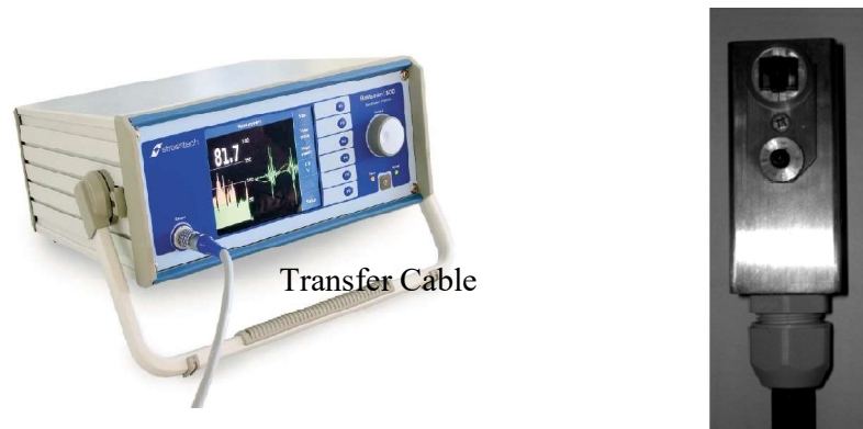
Figure 2.7. Barkhausen Noise analyzer with sensor
