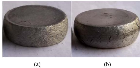
Figure 4 Photograph of the forged alloy A billets (A356 alloy), (a) at 300°C (b) at 500°C (see online version for colours)
