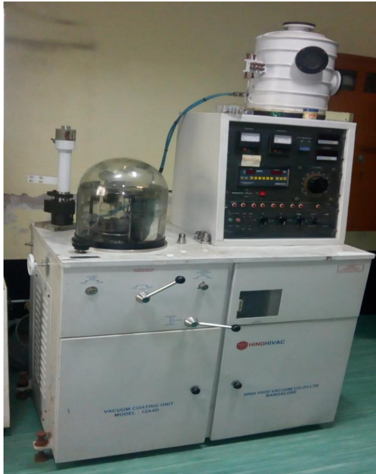
Figure 4.1: Front view of Hindhivac 12A4D thermal evaporator.
