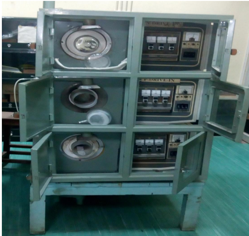
Figure 4.4: Front view of Bench furnace.
