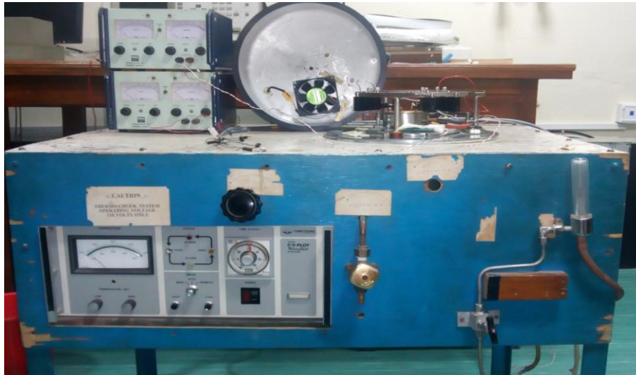
Figure 4.2: Front view of Thermo-chuck-system.
