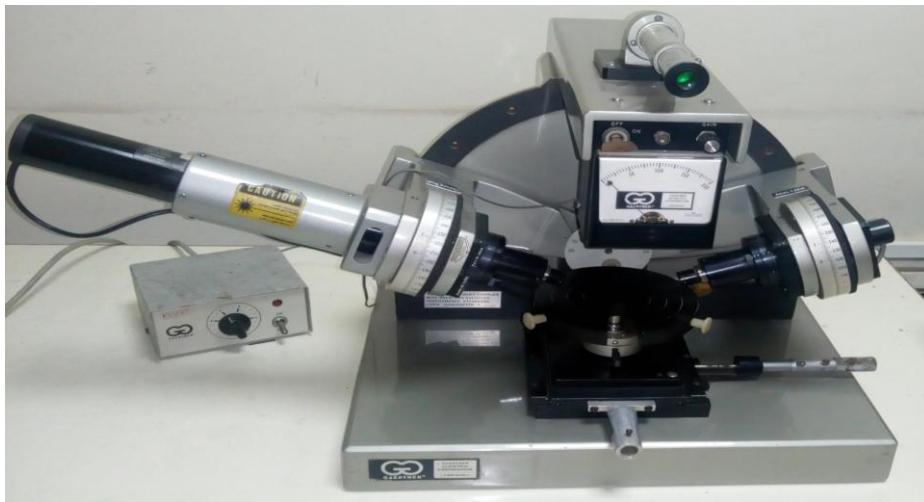
Figure 4.5: Front view of L117 Gaertner Scientific Corporation ellipsometer.
