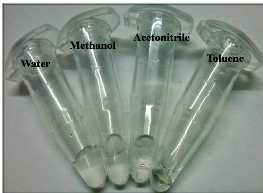
Figure. 3.13. Visual photographs of PdNPs made by using 0.001 \times 10^{-3} M 3-APTMS, 1.9 M Cyclohexanone and 0.005 M K_2PdCl_4 as shown in Table 3.5 (A) and their dispersibility in water, methanol, acetonitrile and toluene.
