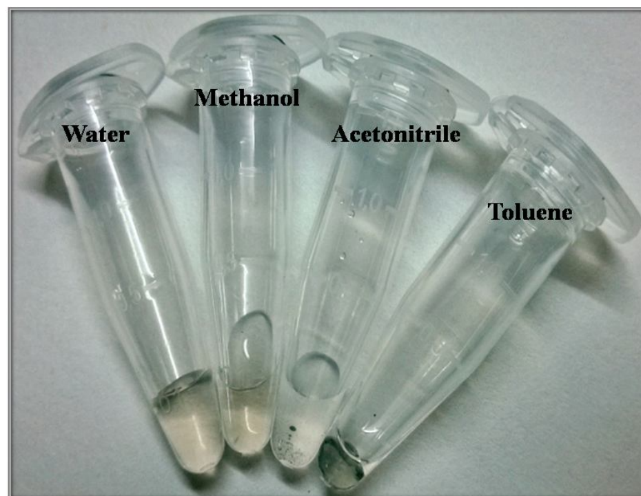
Figure. 3.20. Visual photographs of PdNPs made by using 3-APTMS (0.5 M), THF-HPO (11.4 mg) and K_2PdCl_4 (0.003 M) as shown in Table 3.4 and their dispersibility in water, methanol, acetonitrile and toluene.
