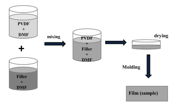
**Figure 2.2:** Hybrid preparation through solution route.
