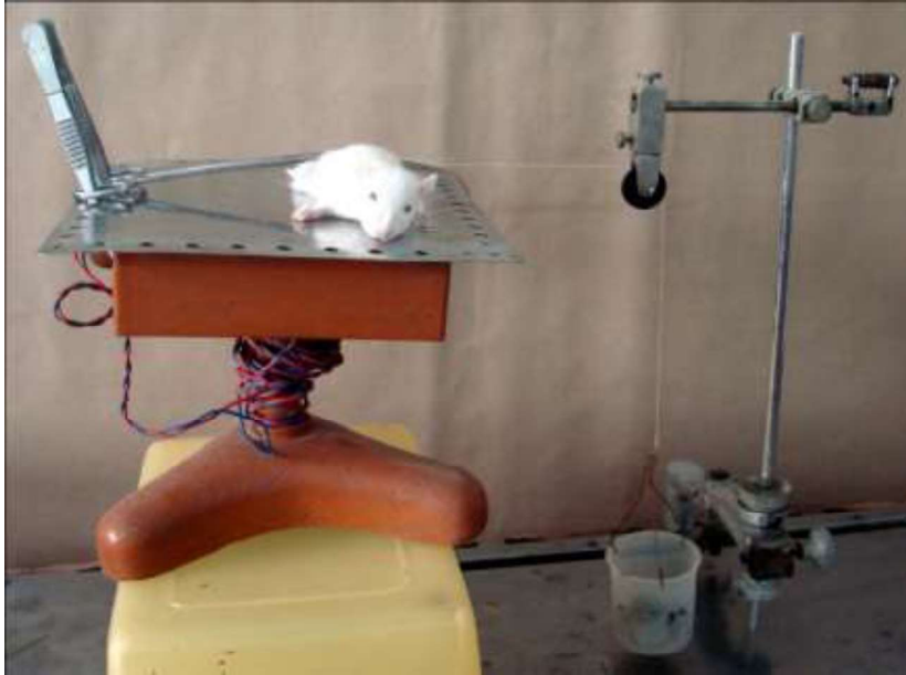
Figure 6: Measurement of wound breaking strength on 10 th day post incision wound by self-made tensometer
