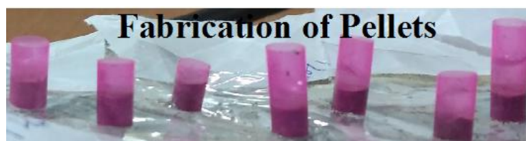
Figure 2.5 Pictorial representation of the fabrication of TiO 2 .cement composite pellets.
