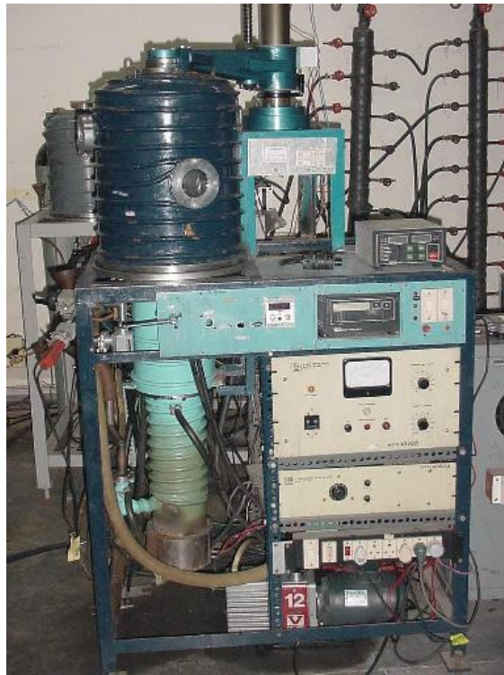
Figure 2.3 Electron beam evaporation unit used for the deposition of TiO 2 film.
