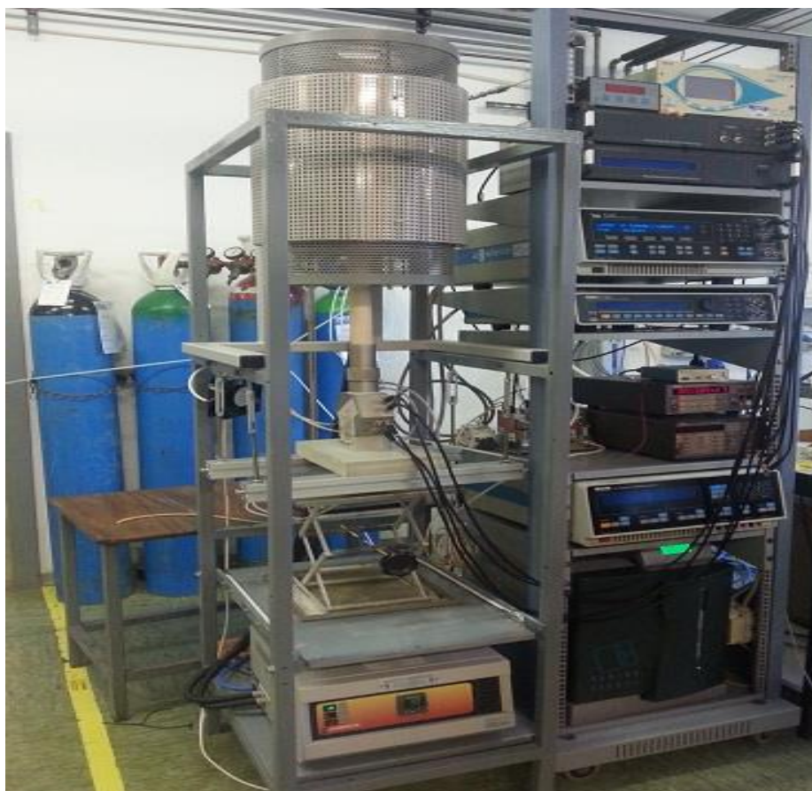
Fig.2.15: The Probostat (Norecs, Norway) system impedance Analyzer (FRA, mod. SOLARTRON 1250 - Schlumberger), in a range of frequency between 10^{-1} - 10^5 Hz.
