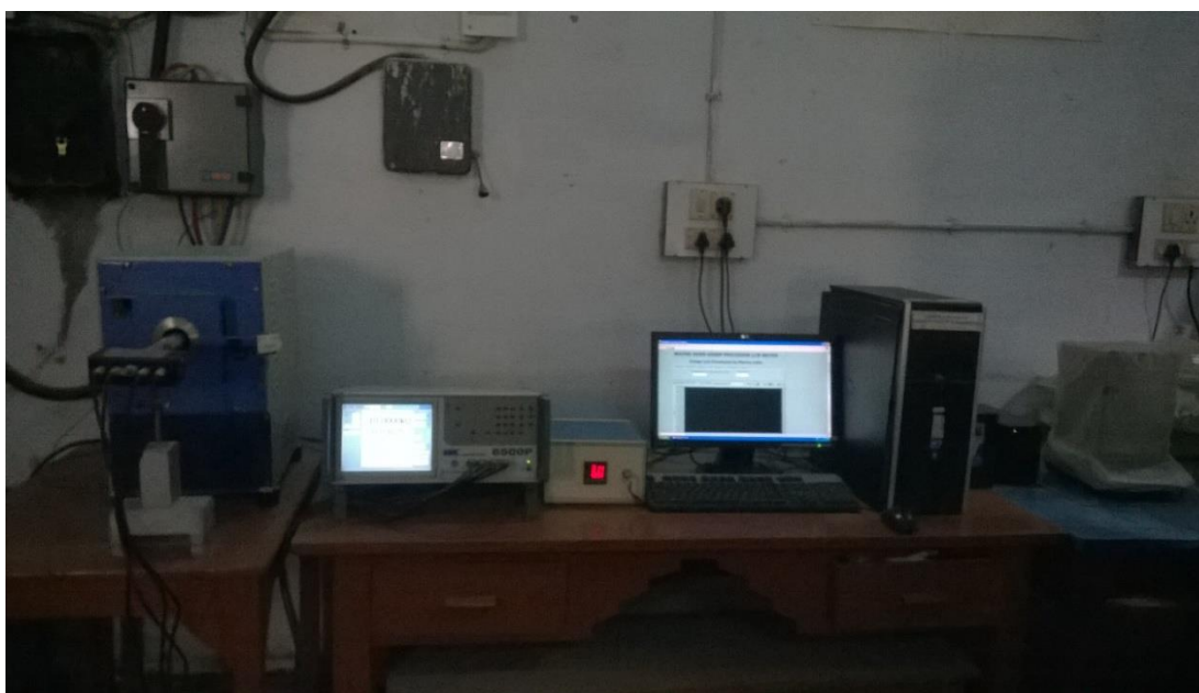
Fig. 2.14: Computer controlled automated impedance analyser setup along with sample holder and furnace (6500 P Wayne Kerr, UK).
