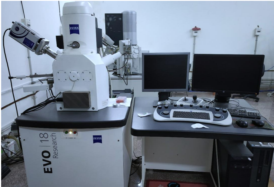
Figure 2.6: Morphological image by Scanninc Electron Microscope [ZEISS EVO 18 SEM].
