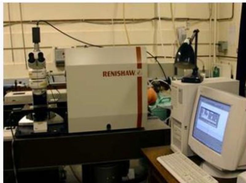
Figure.2.7: Renishaw micro Raman spectroscope.
