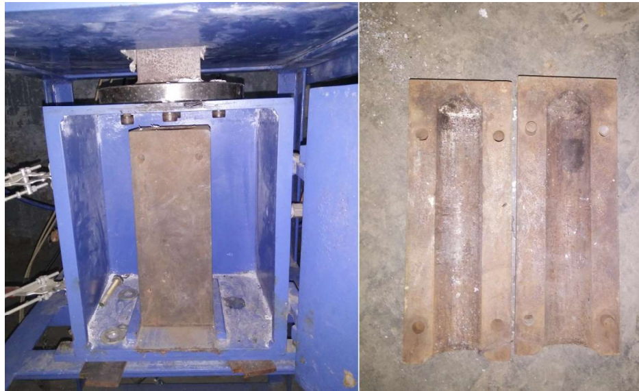
Figure 4. 12: a) Die holder with die b) two-part die of cast iron
