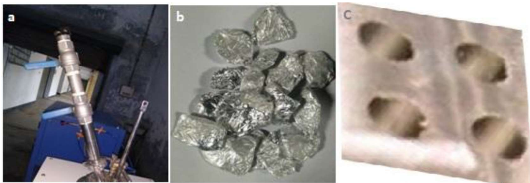
Figure 4. 14: Different modes of reinforcement addition in molten metal a) through anti-chamber b) aluminum foil capsule c) array of the hole
