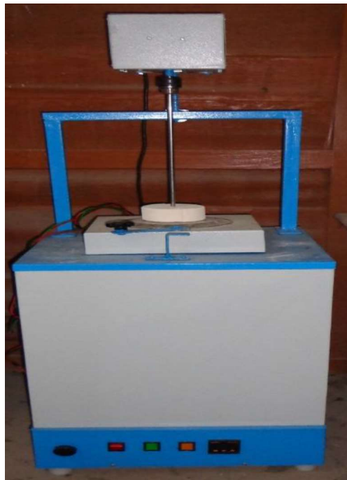
Figure 4. 3: Photograph of first experimental stir casting set-up
