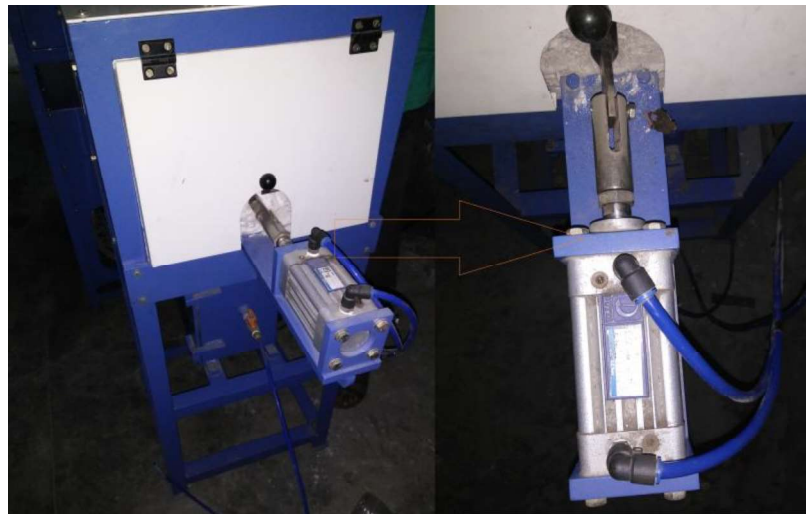
Figure 4. 11: Pneumatic high-pressure cylinder arrangement for opening and closing of the pouring valve
