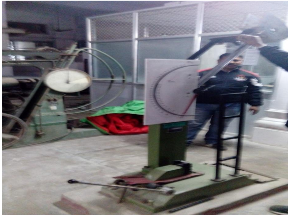
Figure B.7 Set-Up for Charpy Test
