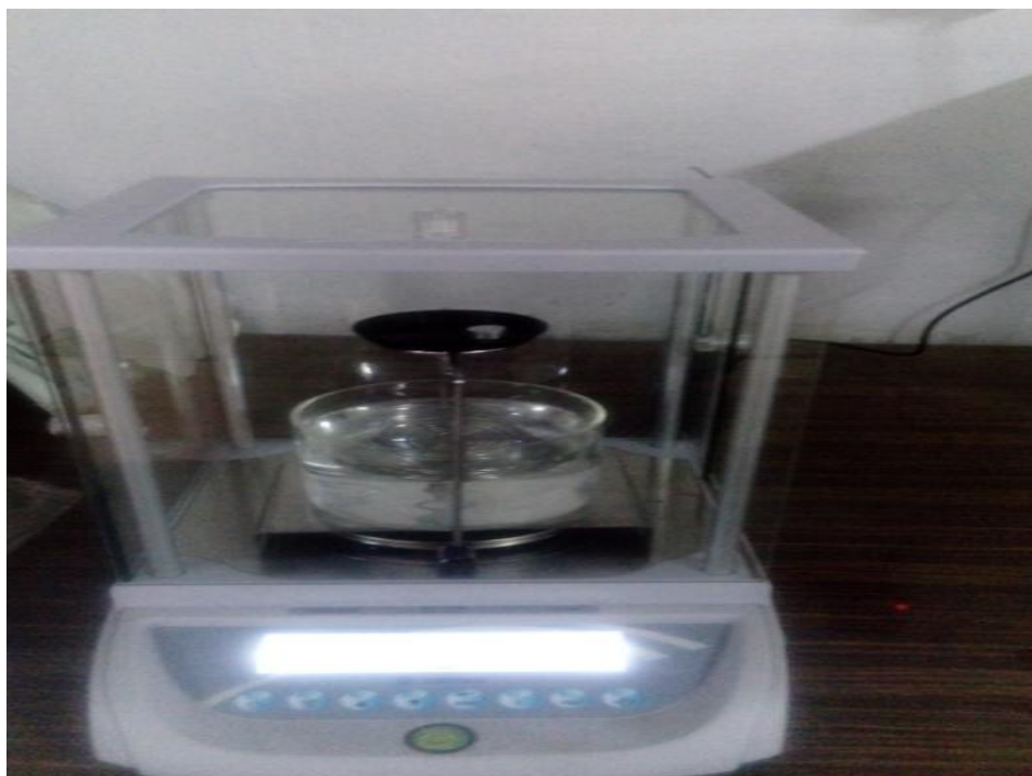
Figure B.4 Density and Porosity Measurement Set-Up
