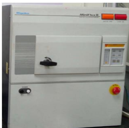
Figure 2.2 The phase formation of prepared samples has been studied by using Rigaku-MiniFlex-II DESKTOP powder X-ray diffractometer with Cu K \alpha radiation ( \lambda = 1.54 \text{ \AA} ) at 30 kV and 15 mA. Crystal structures of each composition were recorded at 2\theta angle between 20 and 80^\circ with a step size of 0.02 . X-ray diffraction analysis revealed all the important parameters such as crystalline structure, lattice parameters, unit cell volume, atomic packing fraction etc.
