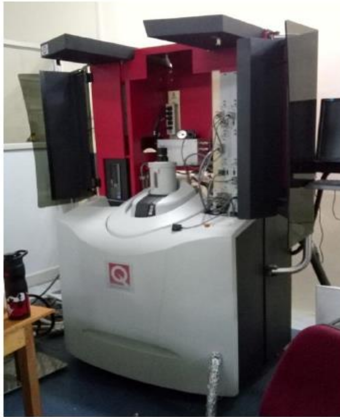
Figure 2.5 MPMS3 set up.
