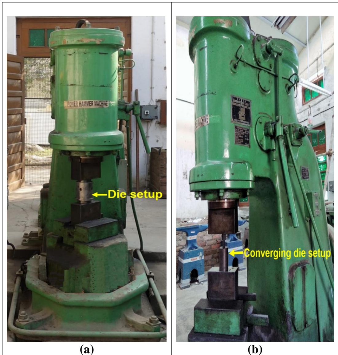
Figure 2.6 Photograph of the Pneumatic Power Hammer with (a) impression die set-ups, and (b) converging die set-ups
