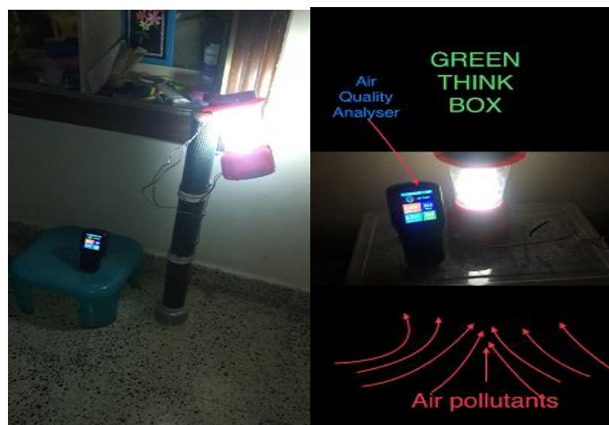
Figure 5.6: Emergency light using standalone type MFC
