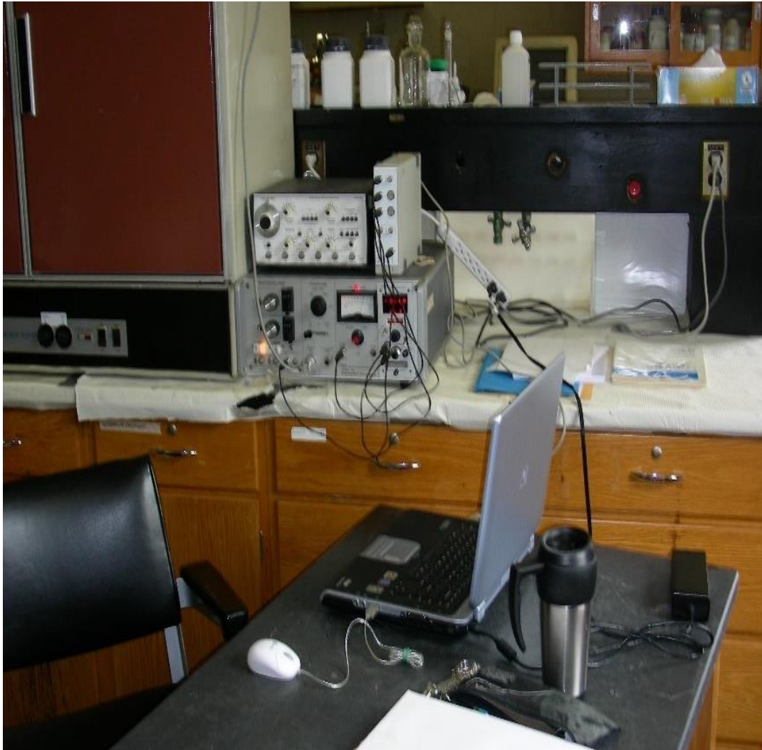
Figure 2.4: Potentiostat and Multimeter with Data Collection System beside Incubator
