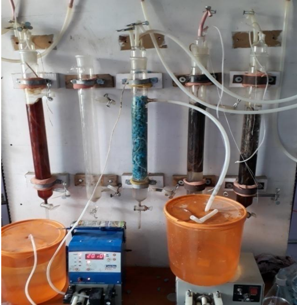
Figure 7(b): Laboratory experimental setup of packed bed bioreactor system
