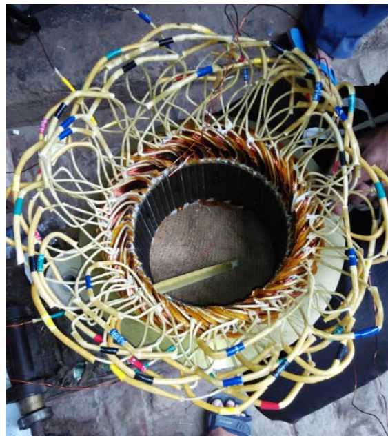
Fig. 3.17 Complete winding connection of outer stator winding
