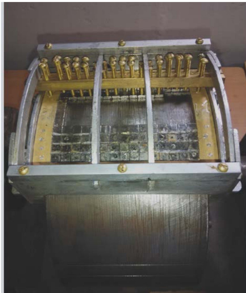
Fig. 3.2. Rotor magnet pasting arrangement of SSFP-PMSG
