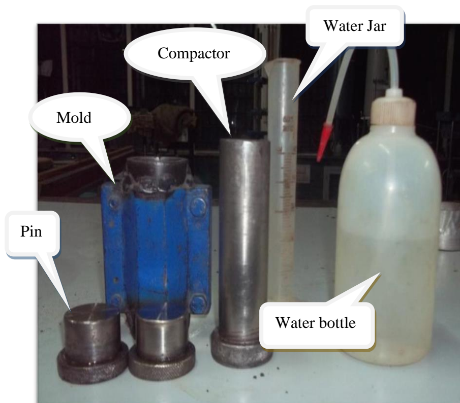
Figure 2.13 UCS mold with accessories
