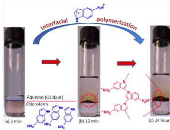
Figure 2.3 Schematic representation of interfacial polymerization of 5-AIn at aqueous/organic solvent system. The top phase is an aqueous solution of APS and bottom phase is monomer/Chloroform solution.
