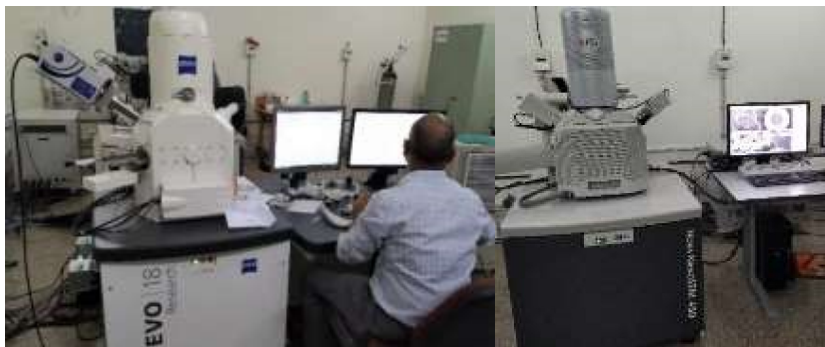
Figure 2.13 Photograph of our SEM and HR-SEM.
