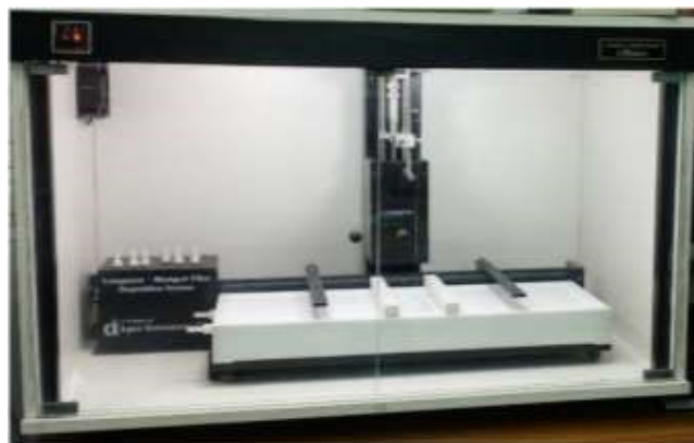
Figure 2.6 Photograph of LB film deposition system.
