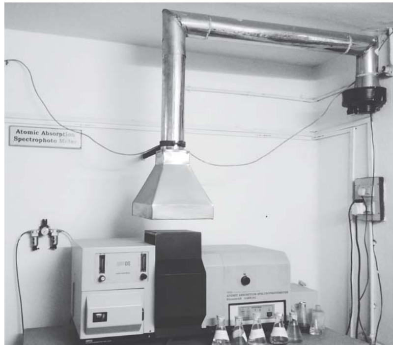
FIGURE 2.11: Atomic absorption spectrophotometer setup (Departmental laboratory, IIT(BHU), Varanasi)
