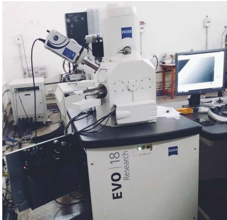
FIGURE 2.10: Scanning electron microscopy with energy-dispersive X-ray spectroscopy detector setup (Departmental laboratory, IIT(BHU), Varanasi)
