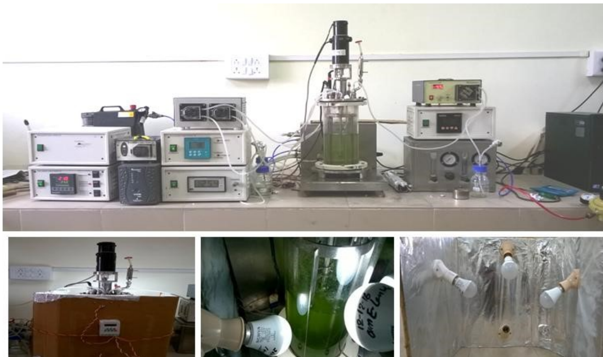
Figure 3.5: Set up of stirred tank photobioreactor
