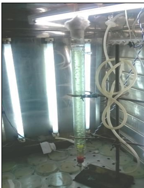
Figure 3.4: The bubble column photobioreactor used for microalgal growth
