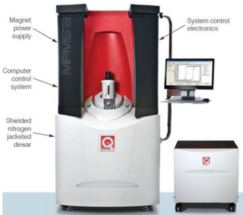
Fig. 3.2.4 MPMS-3, Quantum Design (USA) used for magnetic measurement.
